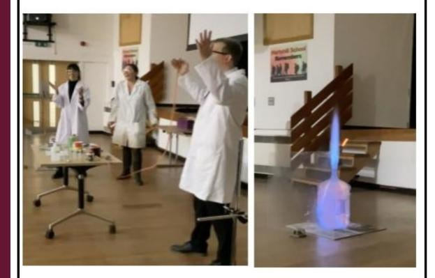
Ethanol was poured and shaken around an empty water bottle. Once removed, the vapours were lit to produce a rocket powered flame!
